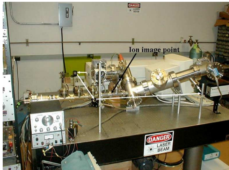
Fig. 1. Picture of the Columbia University LIS on the work bench. The optical path of the Nd:YAG laser has been drawn with white arrows to show where it enters the vacuum system. Except for the pump manifold, the vacuum components on the right, up to the ion image point, are the essential LIS parts to be installed in the accelerator terminal.
