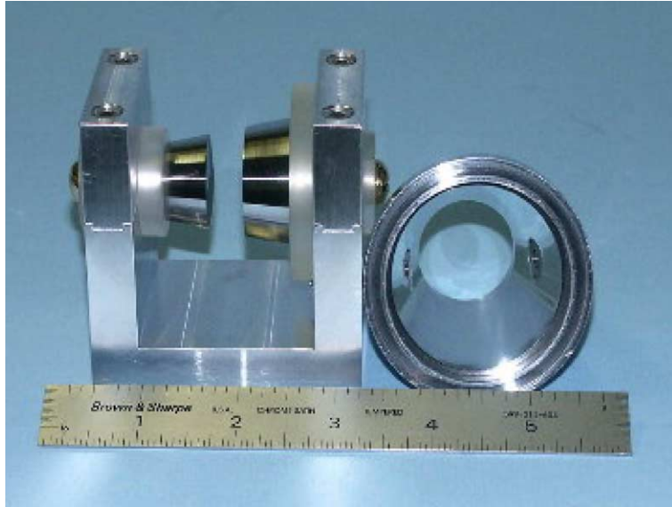
Fig. 3. This photograph of our spherical ESA shows two electrodes and their insulating stand-offs mounted in a U-frame. On the right is a conical sheath that is placed around the electrodes. The sheath is an electrically grounded surface that is used to shape the effective electric field boundary.
