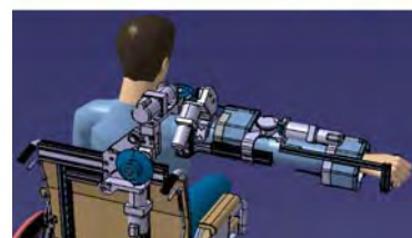
Fig. 5 The gear systems and the arm holders of the exoskeleton
