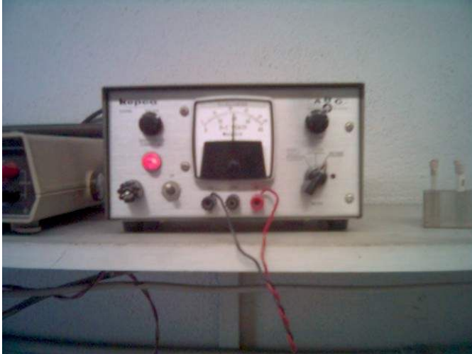
Figure 10: Voltage supply for 60 Hz marginal oscillator.
