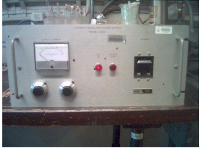
Figure 2: Main magnet power supply. The main power switch is at right; the current knobs and meter are at left.
