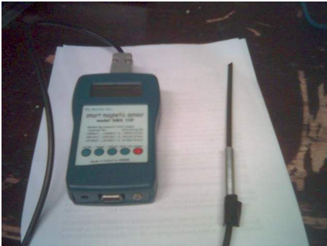
Figure 3: Hall Effect Gaussmeter and field probe. There is also a manual available.
