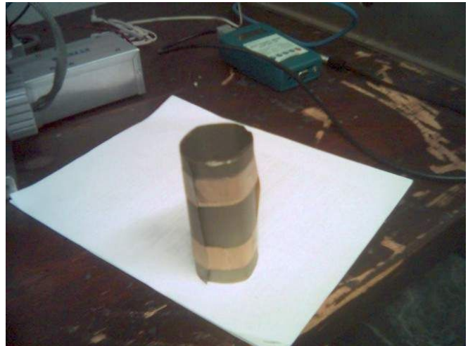
Figure 4: Cylinder of magnetically soft material, used to accurately calibrate the meter to zero field.
